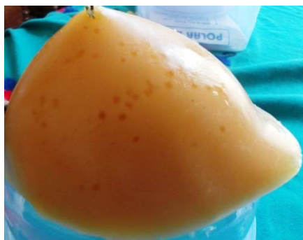
Fig. 1: Bacteriological Gelatin - Based Breast Phantom (Developed in the lab)
