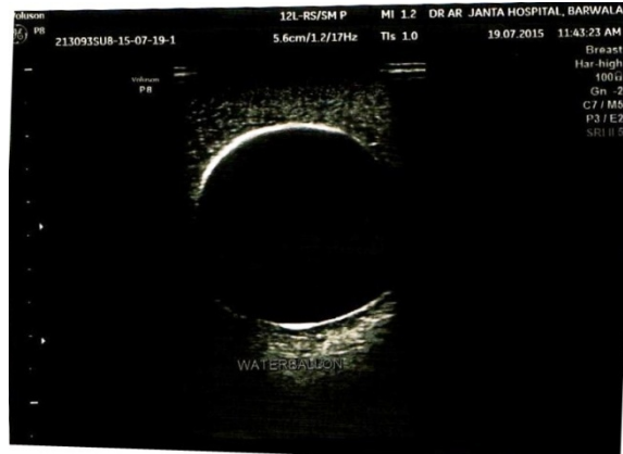
Fig. 5: Sonogram of Water Balloon (mimicked cystic lesion) in phantom (Imaging done at Janta Hospital, Barwala)
